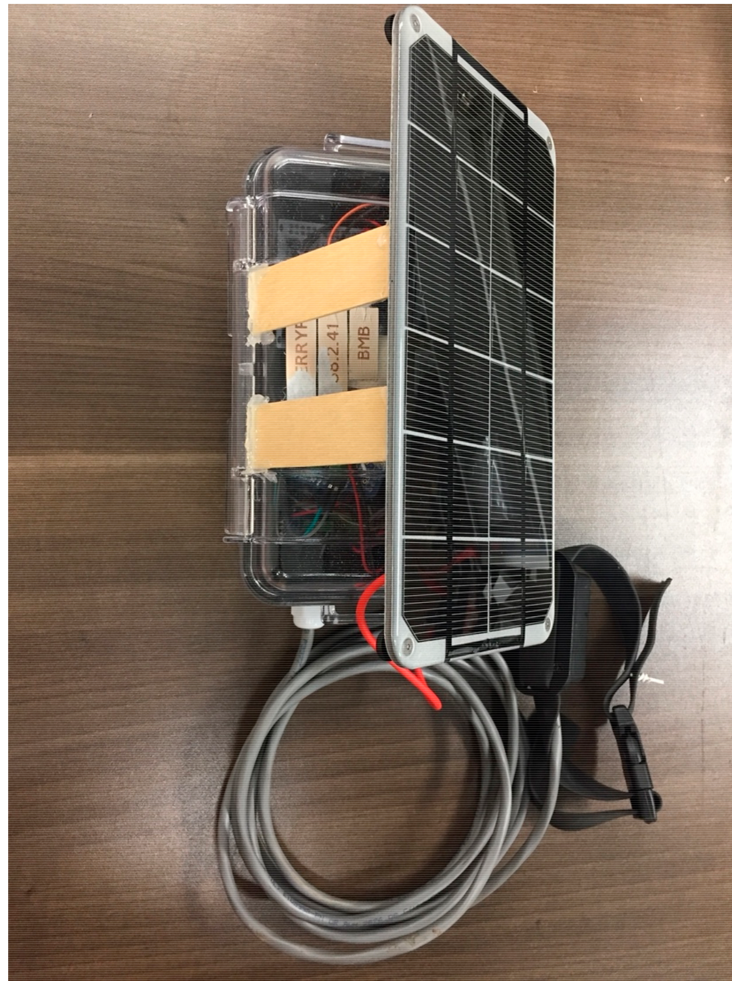
Figure 8. Solar-powered CIWS computational node prototype.
