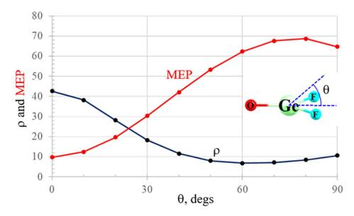
**Figure 3.** Electron density  $(10^{-5} \text{ au})$  and molecular electrostatic potential (MEP)  $(10^{-3} \text{ au})$  of GeF<sub>2</sub>O as a function of the displacement from the molecular plane  $\theta$ , at a distance of 2.5 Å from the Ge atom.
