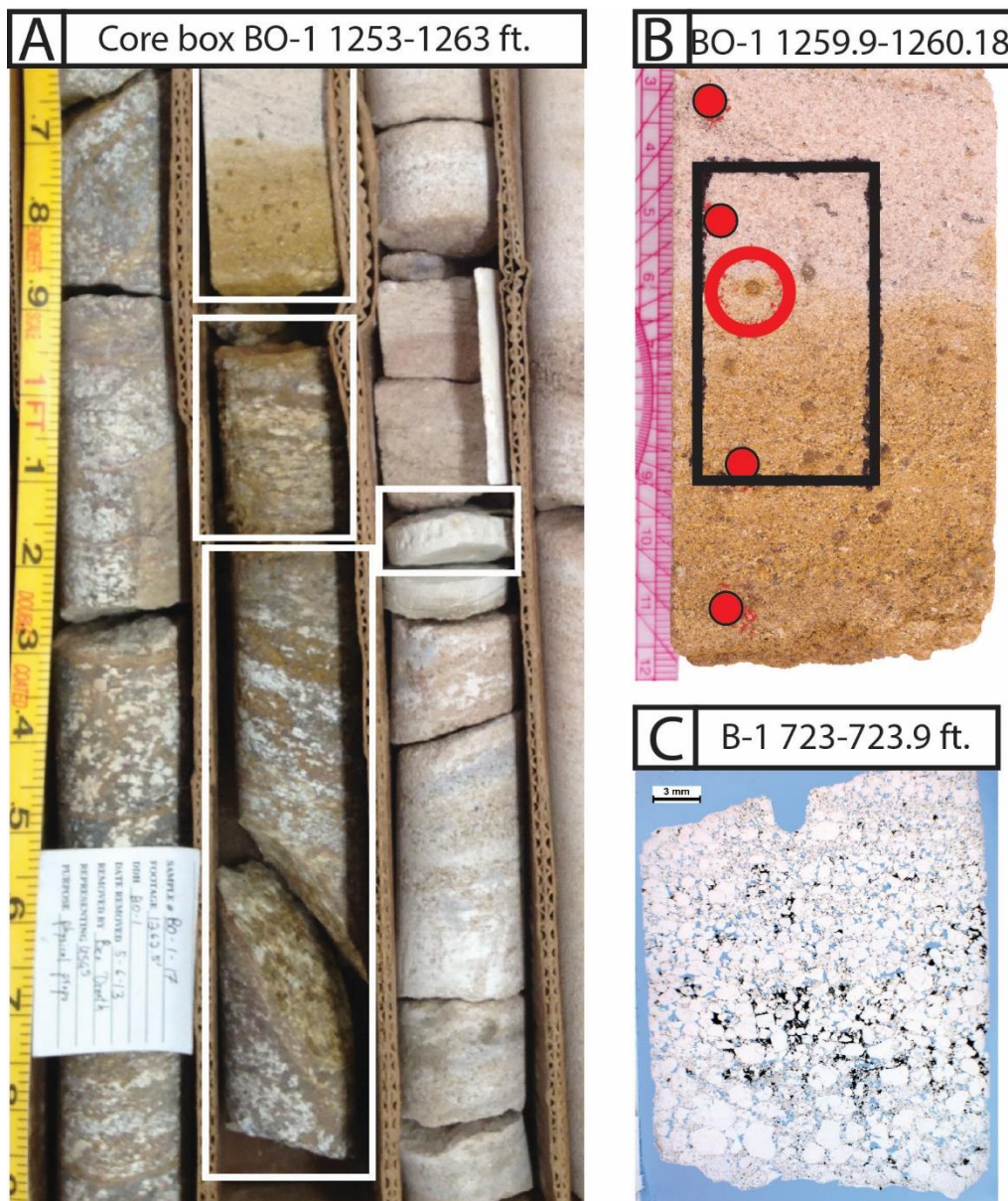
Figure 3: Visual methods summary: A) Individual samples are selected from the drillcore with a focus on changes in lithology, alteration zones, or structural features such as faults, veins, and fractures; B) Locations for thin sections (black rectangle) and relative porosity and permeability testing (red) are noted; C) In addition to petrographic analysis to determine mineralogy, alteration phases, and micro-structures, plane polarized thin sections impregnated with blue fluorescent dye are examined to document pore spaces and fractures.
