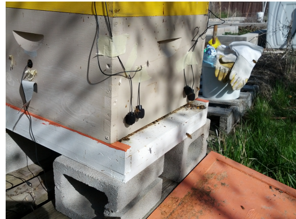
(e) Four microphones hanging near to the beehive entrance
