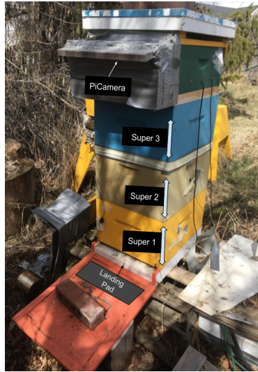
(b) Beehive of 3 supers with BeePi on the top
