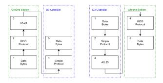
Figure 6: A flow chart showing how data is packaged and transmitted during uplink (left) and downlink (right).
