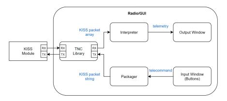
Figure 8: The basic architecture of the D3 Ground Station program. The main GUI is always running and all other processes are handled by threads.
