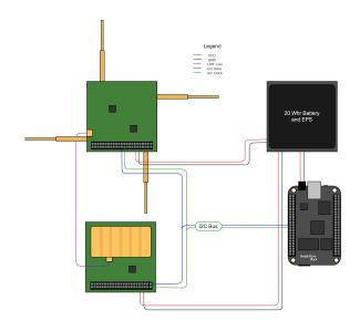
Figure 4: High-level onboard radio hardware schematic.
