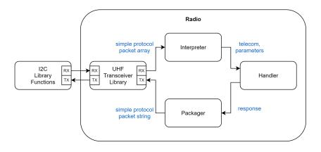
Figure 7: The basic architecture of the onboard radio software. All nodes are implemented as classes. Data flow between nodes is controlled by the Radio class.
