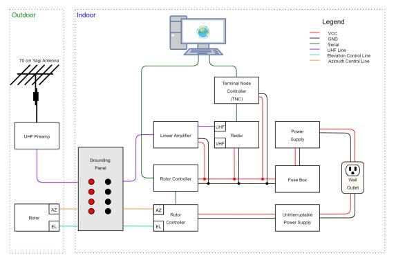
Figure 3: High-level ground station hardware schematic.
