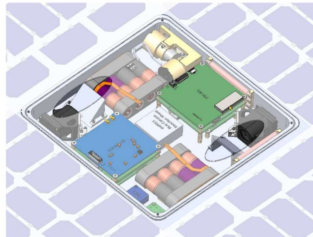
ISARA avionics notional reconfigured into a DiskSat "chassis box"
