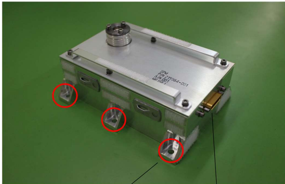
Electrical interface Satellite interface connector mounting holes
