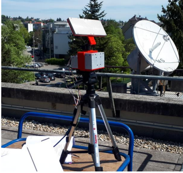
Figure 8: iDRS unit terminal and receiver for the global persistent communications unit hardware in the test-bench
