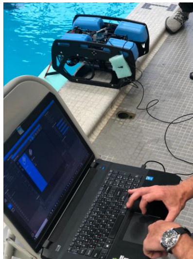
Calibrating onboard sensors for SeaRover pool testing
