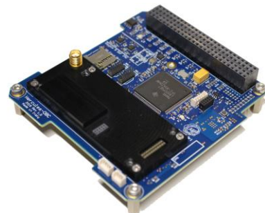
Figure 16: HERCULES OBC with a GAUSS UHF radio fixed to it in the daughterboard slot
