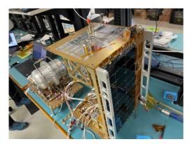
Figure 7: The Halcyon and Primary refueling tank during integration with Tenzing and software checkout.
