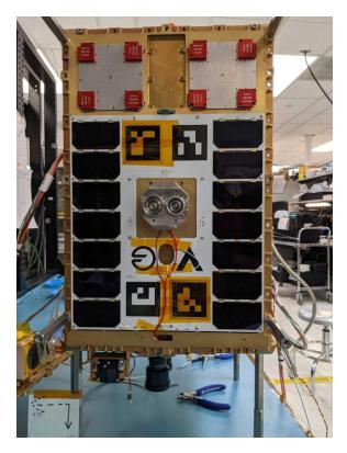
Figure 8: Passive Spark embedded within an Astro Digital smart panel and installed on Tenzing for flight. Kapton tape will be removed before flight
