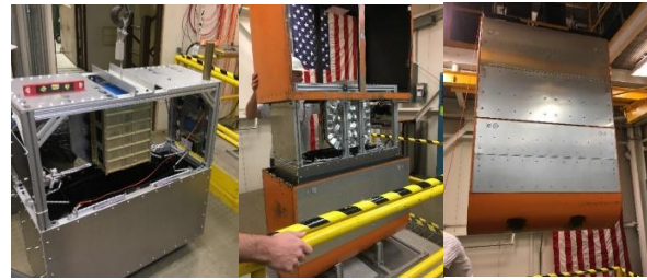
Figures 9, 10, 11: Hoisting Experiment Chassis (left), Encapsulating Experiment Chassis in Drag Shield (Center), Hoisting of Full Rig (right) (5)
