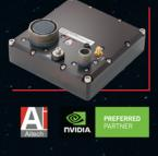
Aitech's A176 Small Form Factor (SFF) AI GPGPU supercomputer with a NVIDIA® Jetson™ System-On-Module will be used for video processing and data recording on NASA's LOFTID.
