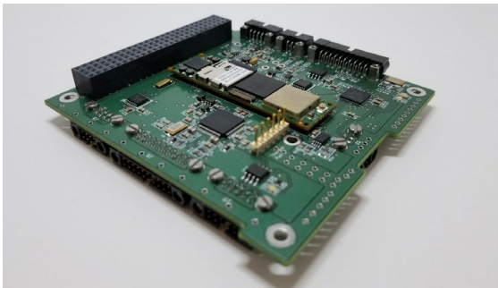
Figure 9: HSFL On Board Computer v3.3 (wifi antenna is not used in-flight version)
