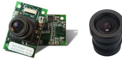
Figure 20: Caspa VL camera, selected as payload for Ke Ao (left). KLB-0360 camera lens included with Caspa VL camera from Gumstix.com (right).
