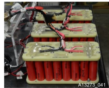
Figure 41: EPL's Li-ion Battery Used in MEP 650 System End-to-End Test
