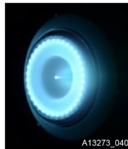
Figure 40: MEP 650 EM2 Operating During End-to-End Testing on Li-ion Battery Power
