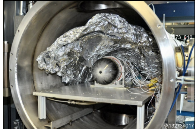
Figure 17: XFS in Tank B Mounted to a Temperature Controlled Plate
