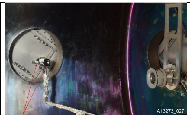
Figure 27: Ion Flux Probe (Left Arrow) and Ion Energy Probe (Right Arrow). EM2 Engine on Far Right.
