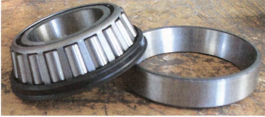
Figure 10: Timkin cup and cone bearings used on the wheel hubs.
