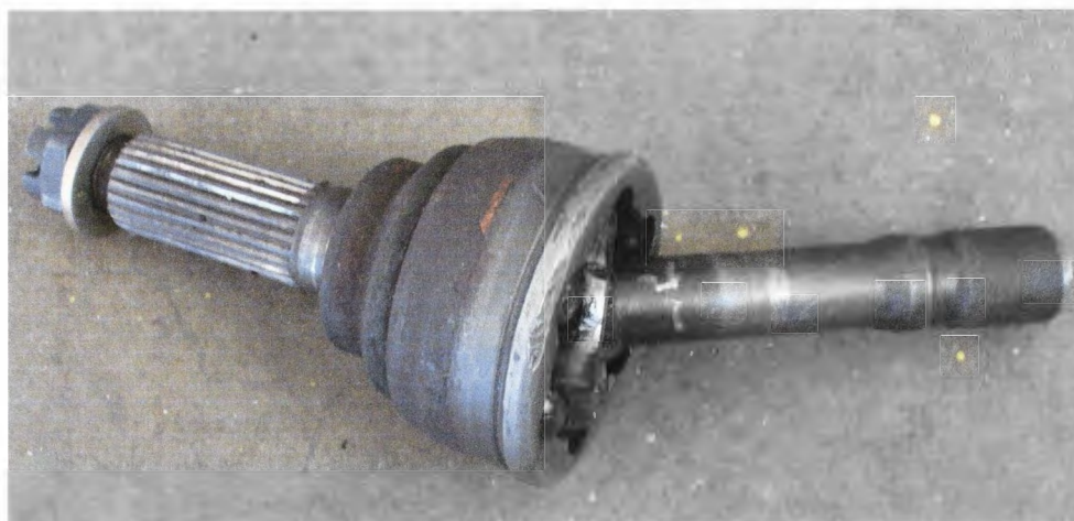
Figure 5: CV joint taken from a Geo Metro.
