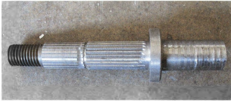
Figure 9: Mandrel made for the machining of the wheel hubs.
