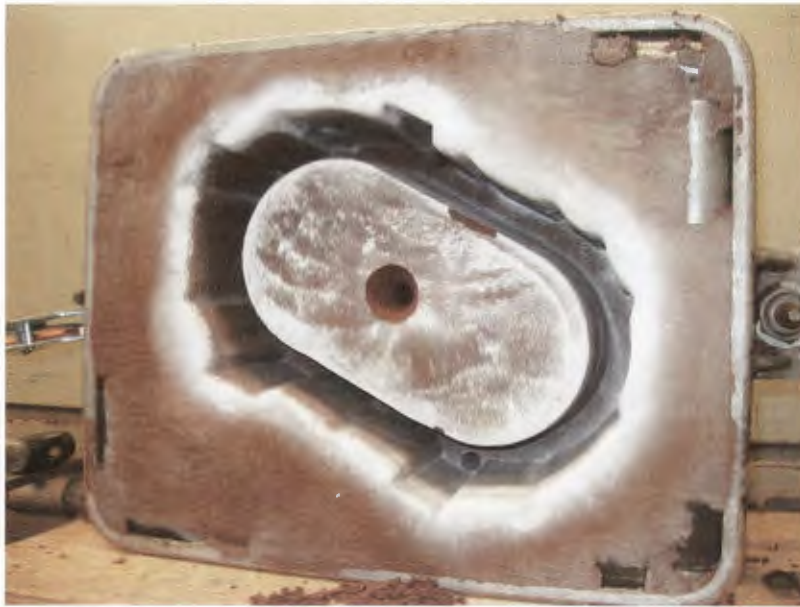
Figure 8: Sand cavity made during the casting of the transmission case.
