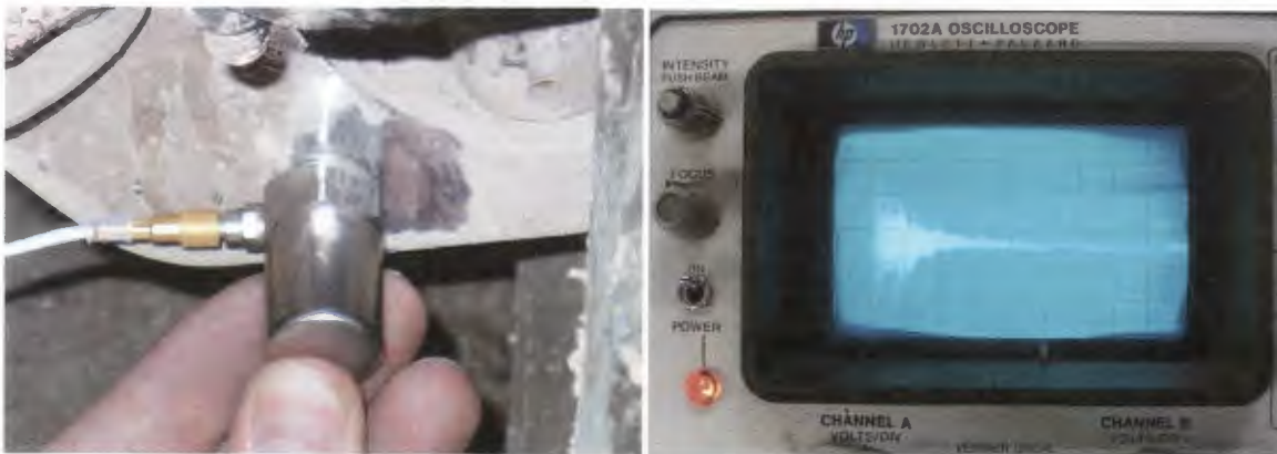
Figure 4: On the left is the accelerometer used to measure the impact on the suspension of the baja, the signal produced by the impact is shown on the oscilloscope on the right.
