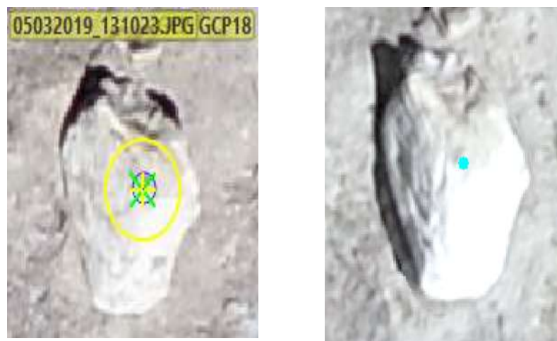
Figure 13. Ground control point selection between the original May, 2019 imagery and a subsequent overflight.
