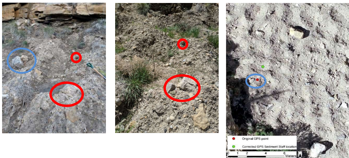
Figure 46. Example of using the ground images and aerial imagery to correlate locations and correct sediment staff GPS points, with red and blue circles corresponding to each other across the images.
