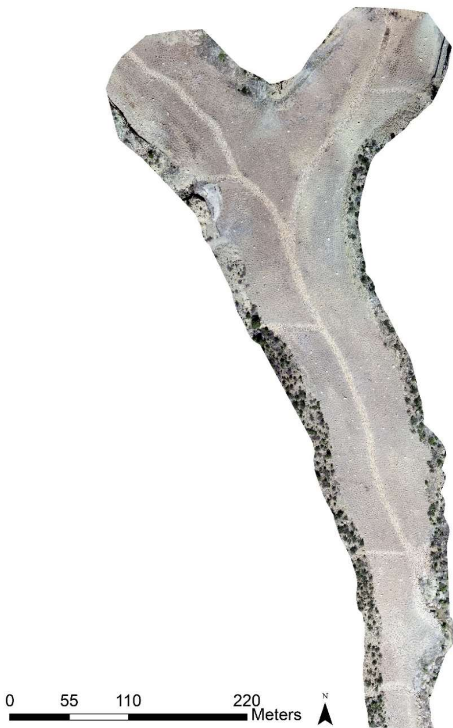
Figure 25. Cottonwood orthomosaic image for May 2019. The northwest arm of the canyon was not covered due to inability to safely collect enough overlapping images of the terrain while avoiding the canyon walls.
