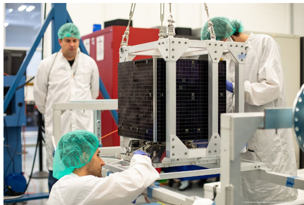
Figure 4: Tetra-1 being assembled by Millennium Space Systems personnel 4
