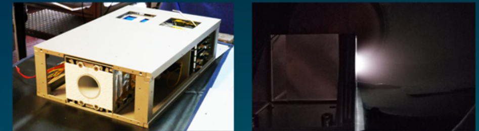
REGULUS integrated in the PoliTo CubeSat Platform (left) and REGULUS fed with iodine under test (right)
