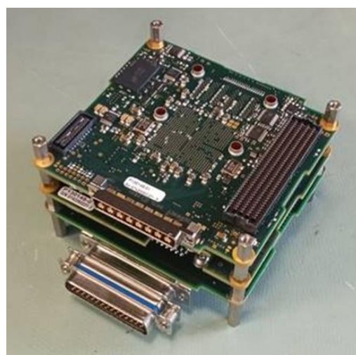
Figure 15. Modular Front End Electronics
