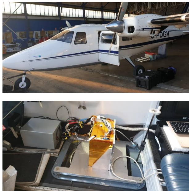
Figure 16. PDG Aviation Vulcanair P68 (Top), EM Camera installed in the aircraft (Bottom)
