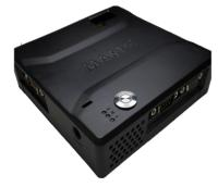
SPiN's MA61C plug-andplay adapter for modular systems with rad-hard LEON-3FT GR712RC processor
