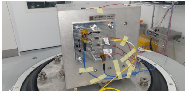
Figure 2: First Generation Optics Module Under Vibration Testing
