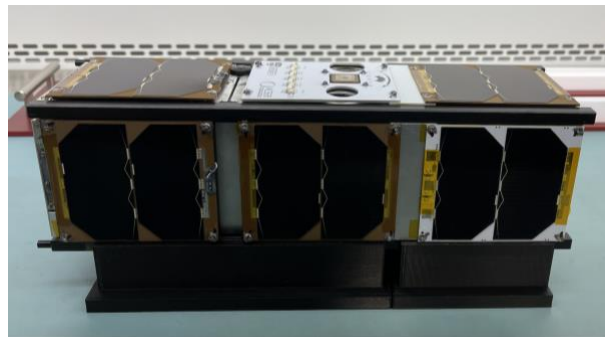
Figure 19 CUAVA-1 after final integration and environmental testing
