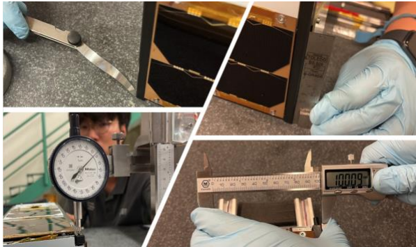
Figure 17 Dimensional measurements during re-integration
