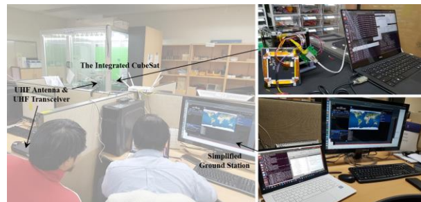
Figure 6: Example of setting for end-to-end and day-in-the life testing
