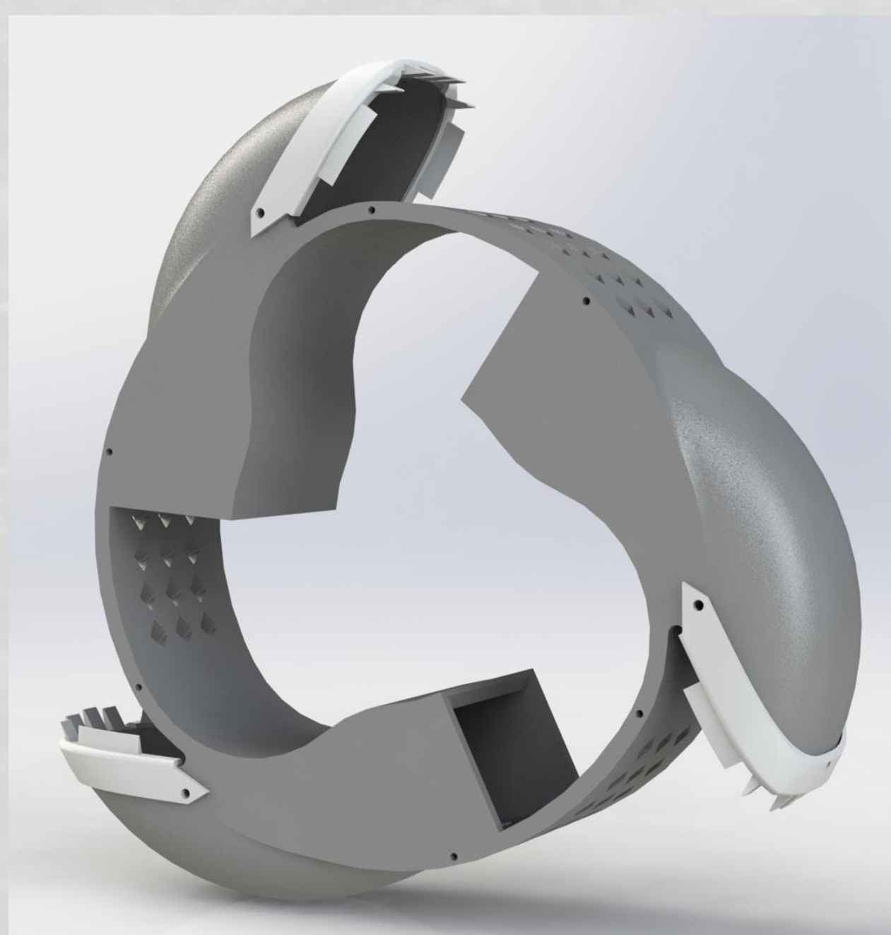
Fig. 2 SolidWorks render of the drum, showcasing rounded scoops, improved filtration, and replaceable scoop teeth
