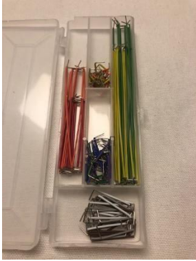
140 pc. Jumper Wire kit, used to wire circuits on your breadboard
