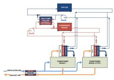
Figure 2: System Diagram (Credit: UFC 3-410-01Appendix F)
