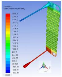
Figure 5: Static pressure of the mixture flow at V=1.86 l/min and ice volume fraction 20% inside the special plate heat exchanger geometry of TTZ Company
