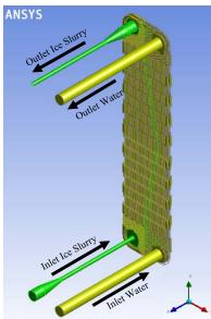
Figure 1: Schematic geometry of special plate heat exchanger for CFD model
