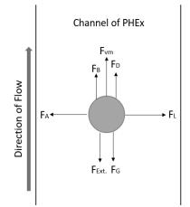
Figure 2: Forces acting on a particle through the channel of plate heat exchanger
