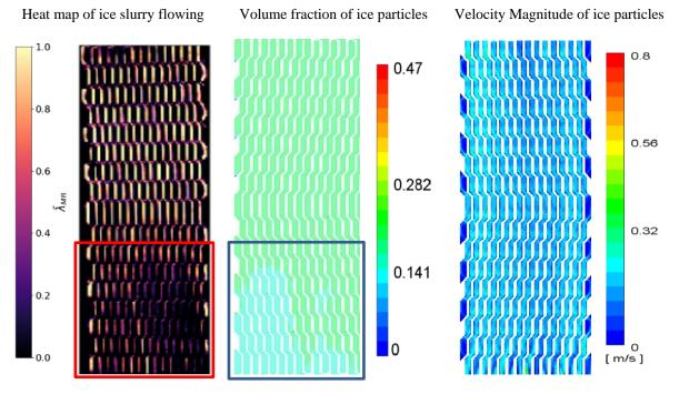
Figure 6: Comparison between the visualization profiles with simulation profiles for ice particles
