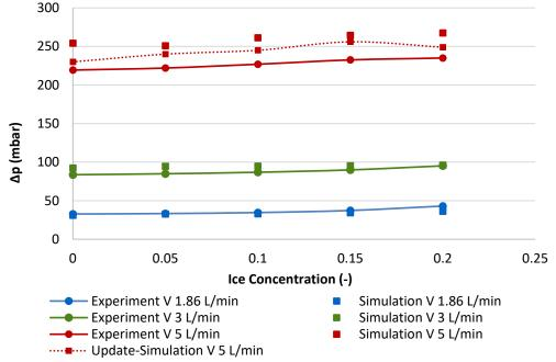
Figure 4: Validation of the pressure drop between experimental and simulation results of the special plate heat exchanger geometry of TTZ Company
