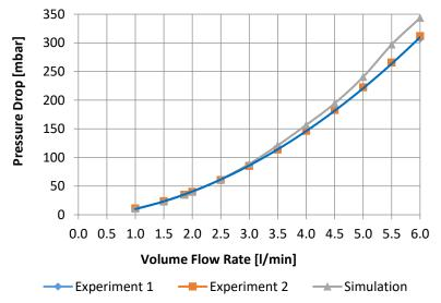
Figure 3: Pressure losses of the single-phase potassium format-water flow as a function of the inlet volume flow in the special plate heat exchanger geometry of TTZ Company
