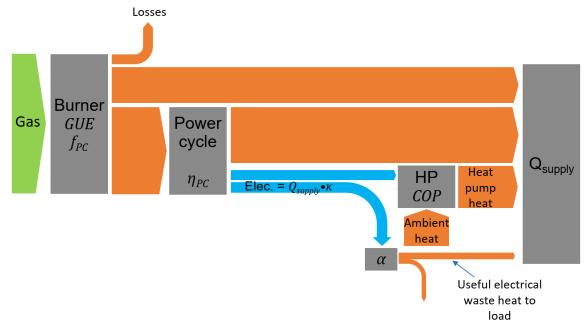
Figure 3: Sankey diagram of energy flows for a generic self-powered heating device, in which only some of the fuel is consumed by the power cycle, some of the electricity produced powers a heat pump, and some of the electrical waste heat is useful.
