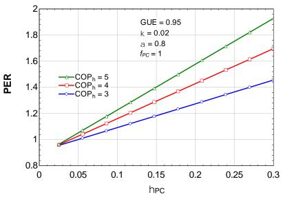
Figure 5: PER as a function of power cycle efficiency for a SPD-HP, with contours for various heat pump COP values.
