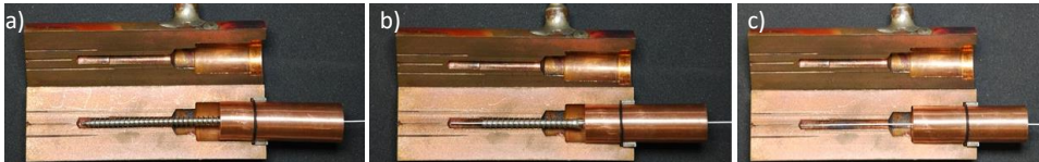
Figure 6: Various penetration depths of the screw
