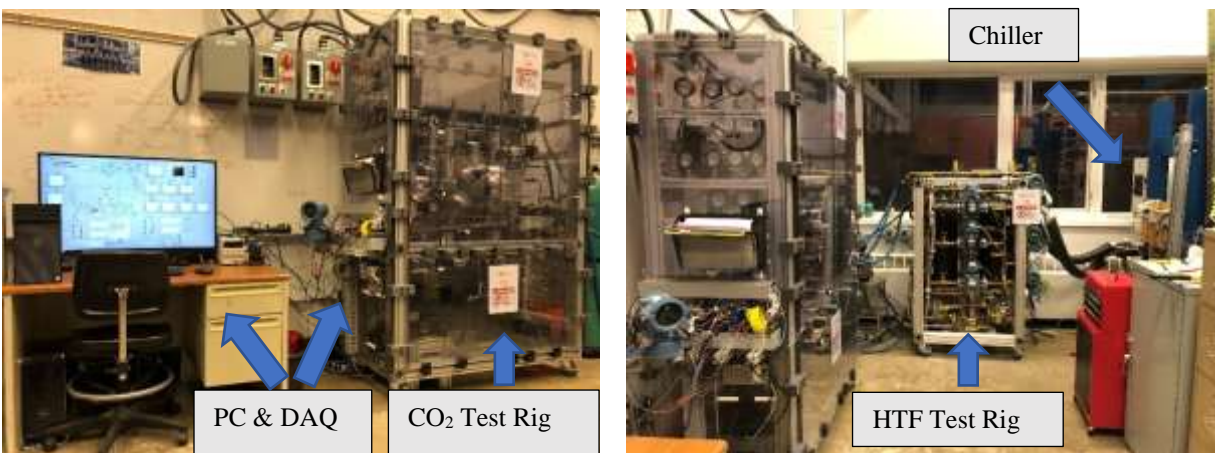
Figure 5: Front and side views of the experimental test rig. The front view shows the CO 2 test rig with the data acquisition and PC. The side view shows the HTF test rig connected to both the chiller and the CO 2 test rig from the right side and left side, respectively.
