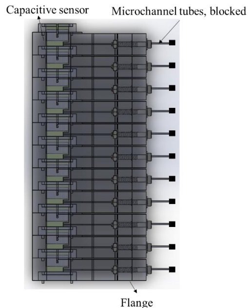
Figure 8: Header assembled from individual partitions
