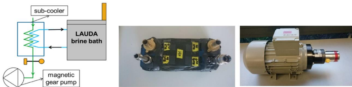
Figure 3: Brazed plate HX (brine refrigerant) for subcooling and magnetic coupled gear pump
