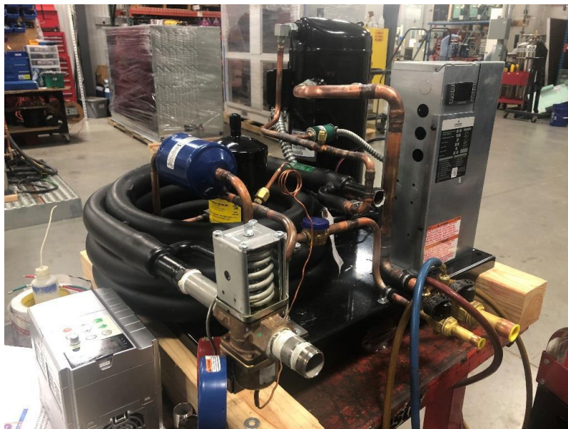
Figure 3: Prototype Unit Compressor and Water-Cooled Condenser Assembly
