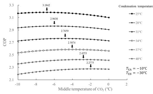
Figure 2: COP versus middle temperature of CO<sub>2</sub> at different condensation temperature
