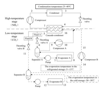
Figure 1: Schematic diagram of the CO<sub>2</sub>/NH<sub>3</sub> cascade refrigeration systems for two temperature ranges
