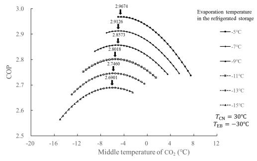
Figure 3: COP versus middle temperature of CO<sub>2</sub> at different evaporation temperature of refrigerated storage
