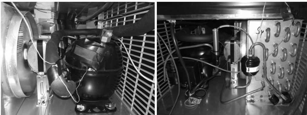
Figure 4: thermocouples at different points on the machine
