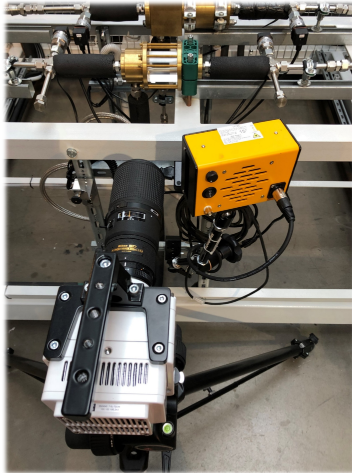
Figure 4: High-speed camera and led lights arrangement
