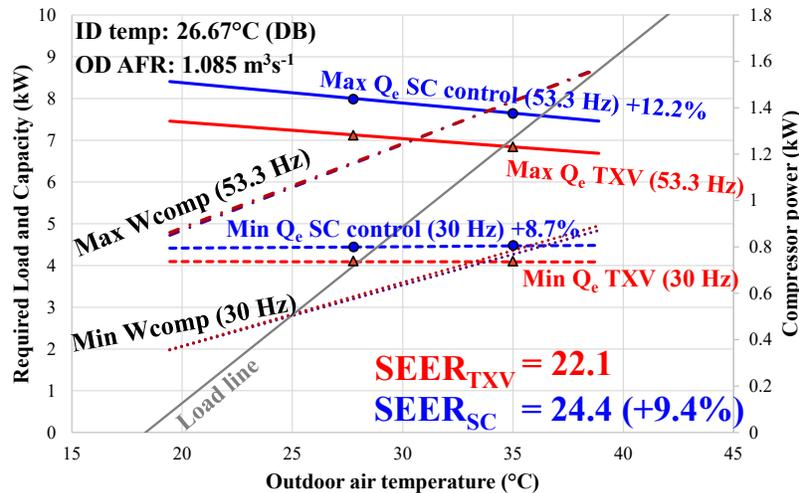
Figure 10: Load, capacity and compressor power vs outdoor air temperature for SEER representation
