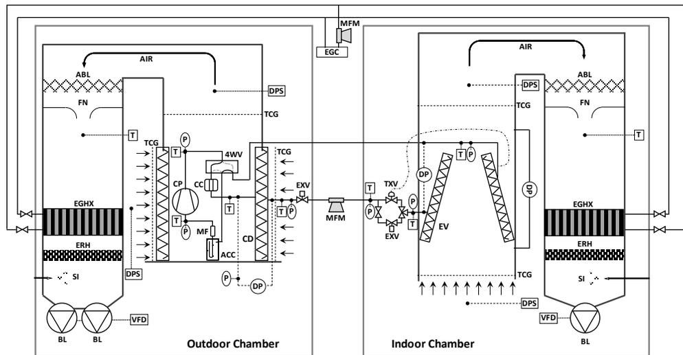
Figure 6: Layout of facility for performance evaluation
