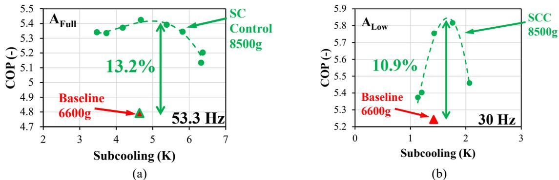
Figure 8: Subcooling control and TXV-based system performance at condition  $A_{Full}$  (a) and  $A_{Low}$  (b)
