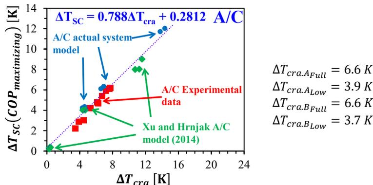
Figure 11: Control curve based on linear regression of the COP-maximizing subcooling as a function of  $\Delta T_{cra}$  and values for SEER points
