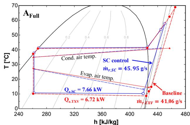
Figure 9: T-h diagram comparing SC control and TXV-based system performance in  $A_{Full}$  condition
