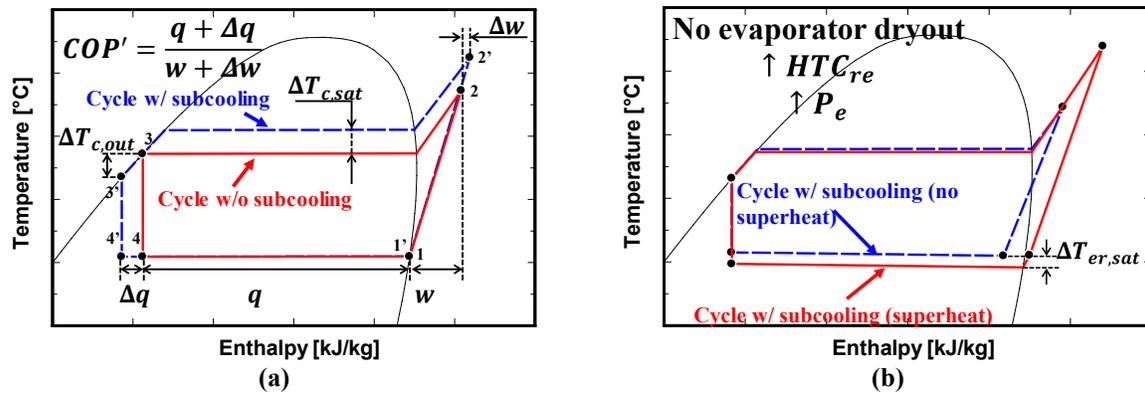
**Figure 1:** Maximum COP as a balance of  $w$  and  $q$  increase with subcooling (a) and increased evaporator effectiveness when operating with no superheat and controlling expansion device through subcooling
