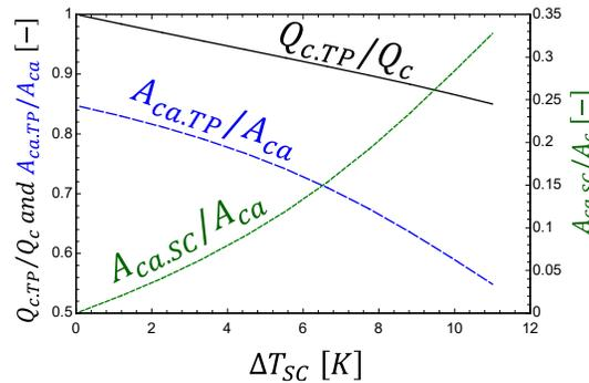
**Figure 2:** Normalized subcooling/two-phase heat transfer areas and two-phase heat transfer vs condenser subcooling
