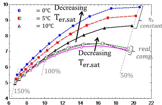
**Figure 5:** COP-maximizing subcooling vs  $\Delta T_{cra}$  for ideal and real compressor curves
