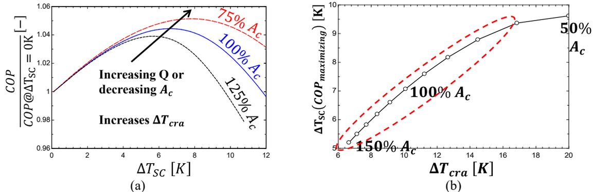
**Figure 4:** Normalized COP vs. subcooling (a) and COP-maximizing subcooling vs  $\Delta T_{cra}$  (b)
