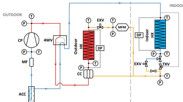
Figure 7: Schematic drawing of the air-conditioning system evaluated
