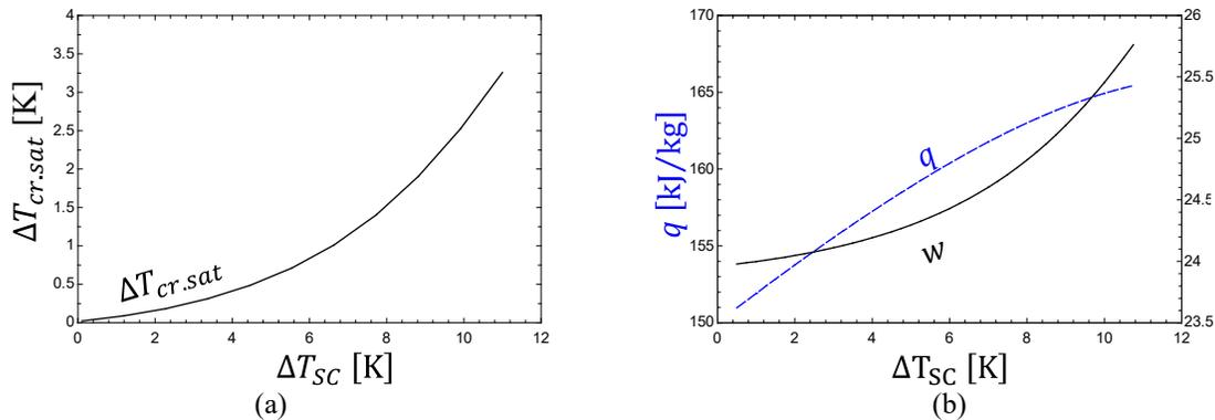
**Figure 3:** Condensation-air inlet temperature difference (a); specific cooling capacity and compressor work (b) vs condenser subcooling
