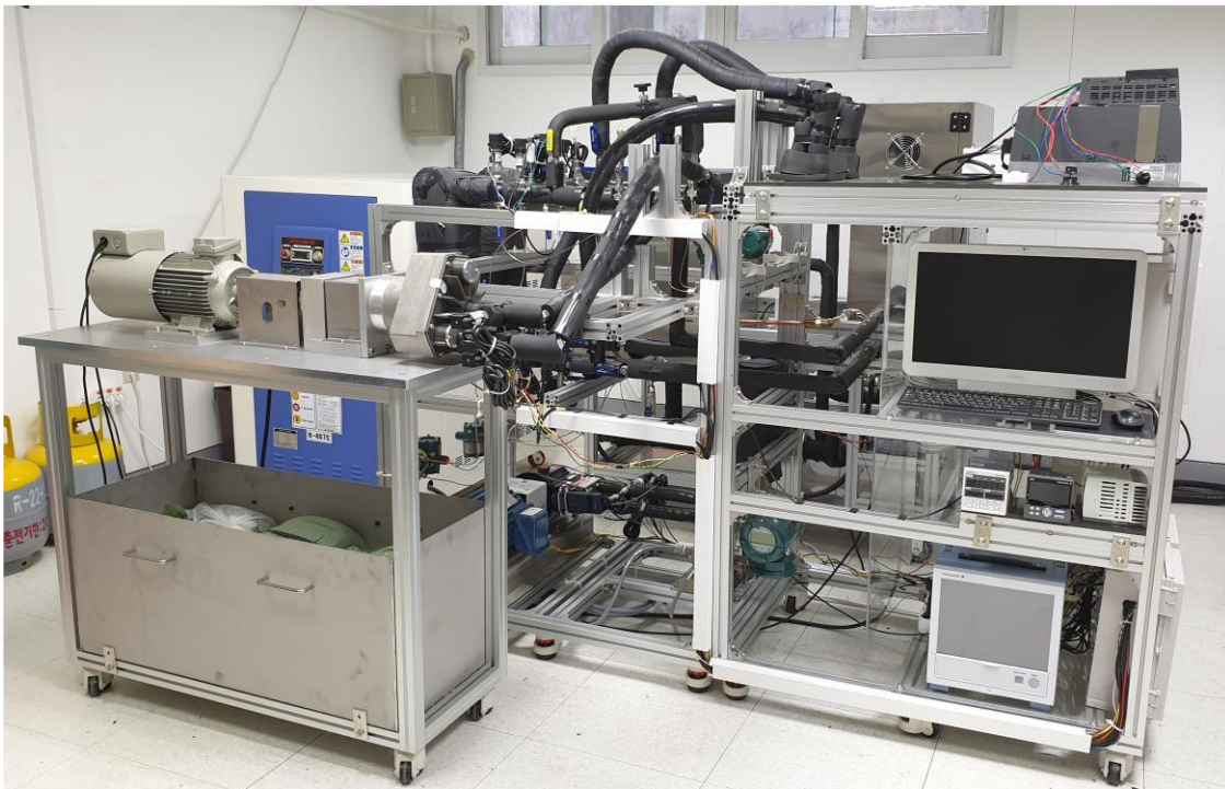
Figure 1: Photograph of the 1 kW lab-scale ORC testbed
