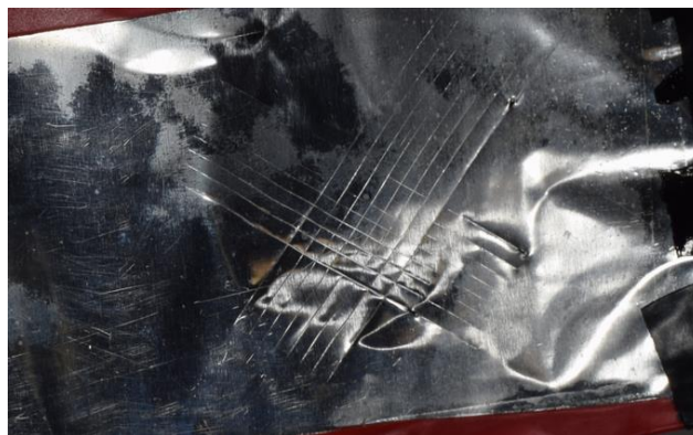
Figure 7: Adhesive testing on coated coupon
