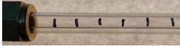
Figure 9: “Sewer situation” refrigerant flow, where liquid refrigerant seems to stand at the bottom of the tube without moving during the transient period.
