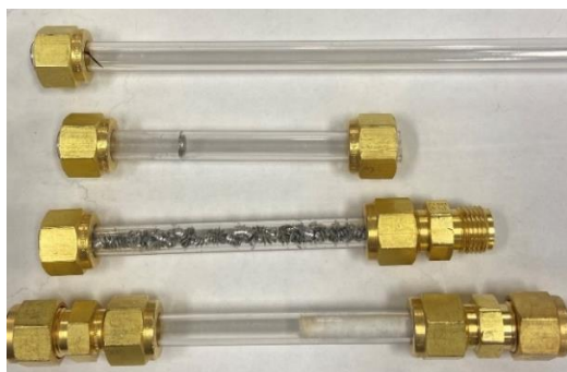
Figure 5: Tube insertion specimens tested. From top to bottom: No insertion, stainless steel disc, dense shavings, and felt.
