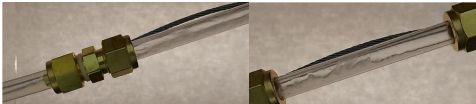
Figure 8: (left) Refrigerant behavior immediately upon compressor startup (right) Observed “wave-like” behavior moments after initial startup.
