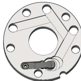
Figure 9 : The discharge gas flow path of the discharge valve on partition plate
