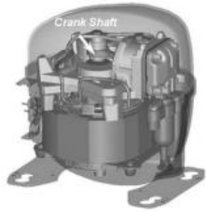
(a) Reciprocating compressors (b) A quarter car model of compressor assembly and its decomposition
