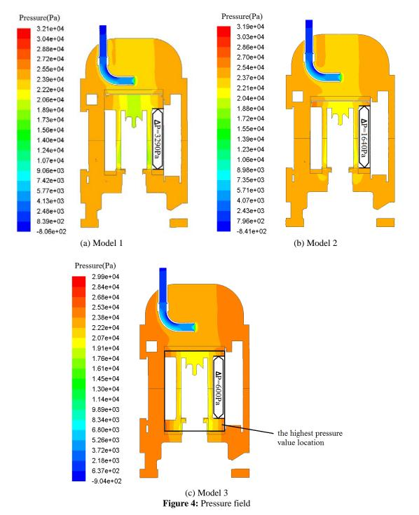
To obtain the lower pressure difference between the motor rotor channel inlet and outlet, the pressure field should be designed. The pressure field determines gas flowing mode and direction, which greatly affects the OCR of the compressor. So not only the compressor parts need to be designed, but also the pressure field in the compressor need to be designed.
