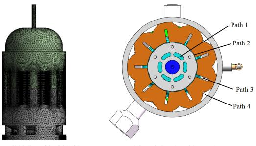
Figure 2: Mesh model of Model 1
