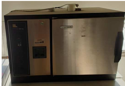
Figure 1: Regulated oven in order to heat the stators up to 200°C.
