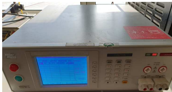
Figure 2: Electrical Safety Tester for Hi-pot (Dielectric Strength) Measurement
