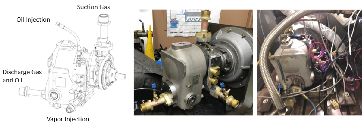
Figure 1: The experimental screw compressor showing suction, discharge, oil injection, and vapor injection
