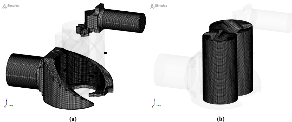
Figure 2: Ports and rotor meshes
