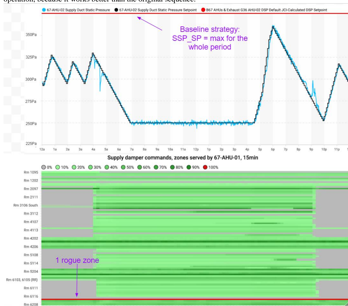
Figure 7: Example of 1 rogue zone (lower panel) driving the original SSP_SP setpoint to remain at 373 pa for the entire day (upper panel, in red), while the new strategy generates lower SSP_SP.
