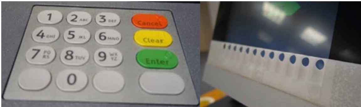
Figure 5.1: The traditional ATM pad and the prototype tactile strip marker for touchscreens (Jokisuu et al., 2016).
