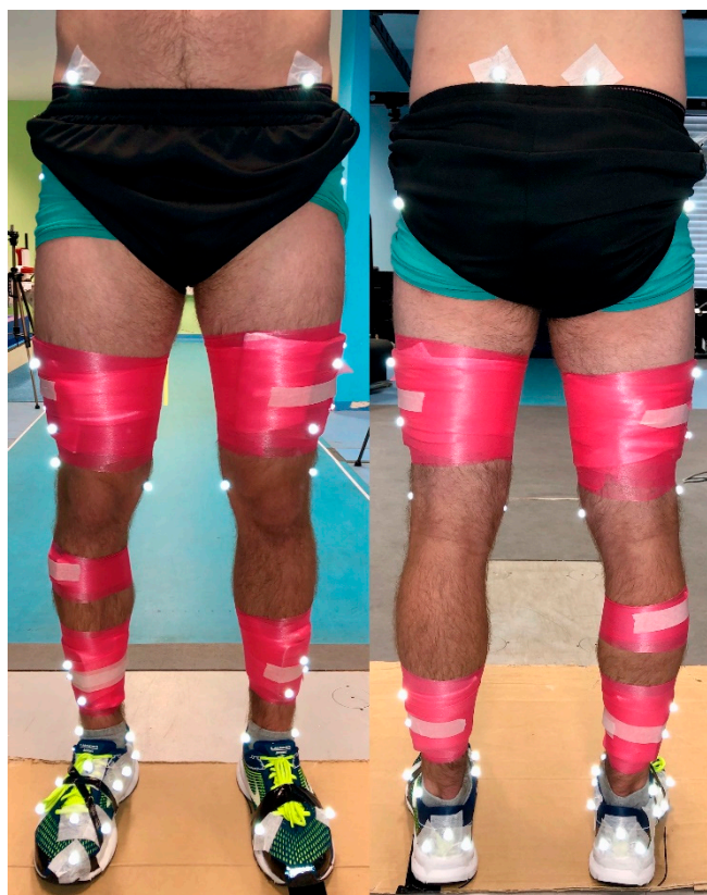
Figure 2. Reflective calibration and tracking markers placement and EMG sensors placement for biomechanical analysis.
